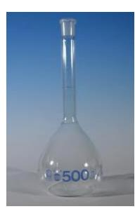
The first thing you'll notice about a volumetric flask, is that it only has a single volume indicated. It is indicated by a line somewhere in the neck of the flask. When you make a solution, you first add your solute, and then carefully add your solvent, so that the solute is dissolved, and for an aqueous solution, the bottom of the meniscus is just touching the line. This means that you've made a solution that's exactly the volume written on the flask.
